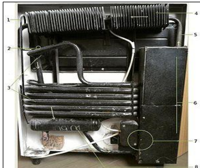
Fig9: Back side photo of a domestic absorption refrigerator.
